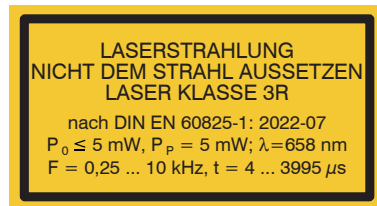
Fig. 4 Laser labels on the sensor cable
