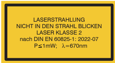
Fig. 1 Laser labels on the sensor cable
