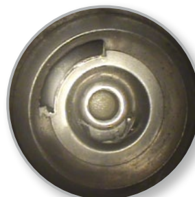
Checking brake cylinder for burrs
