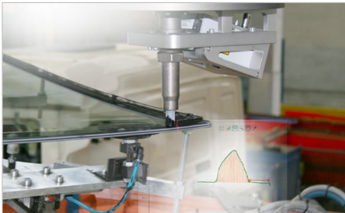
Inspection of the adhesive beading
