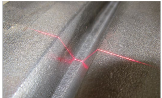
V-seam measurement on pipes
