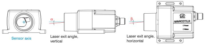
Abb. 9 Manufacturing tolerance laser exit versus sensor axis
