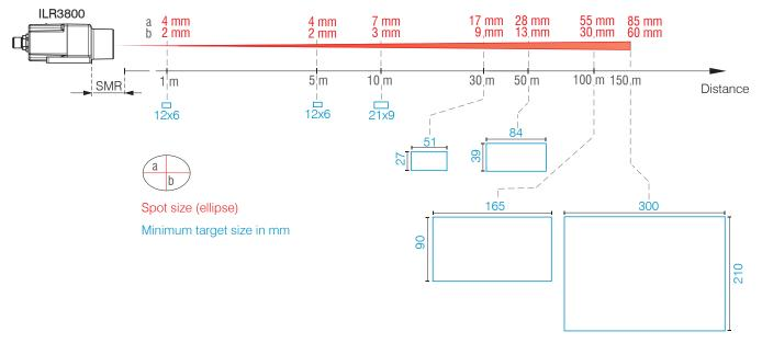
Abb. 4 Laser spot dimensions and size of measuring object depending on the distance
