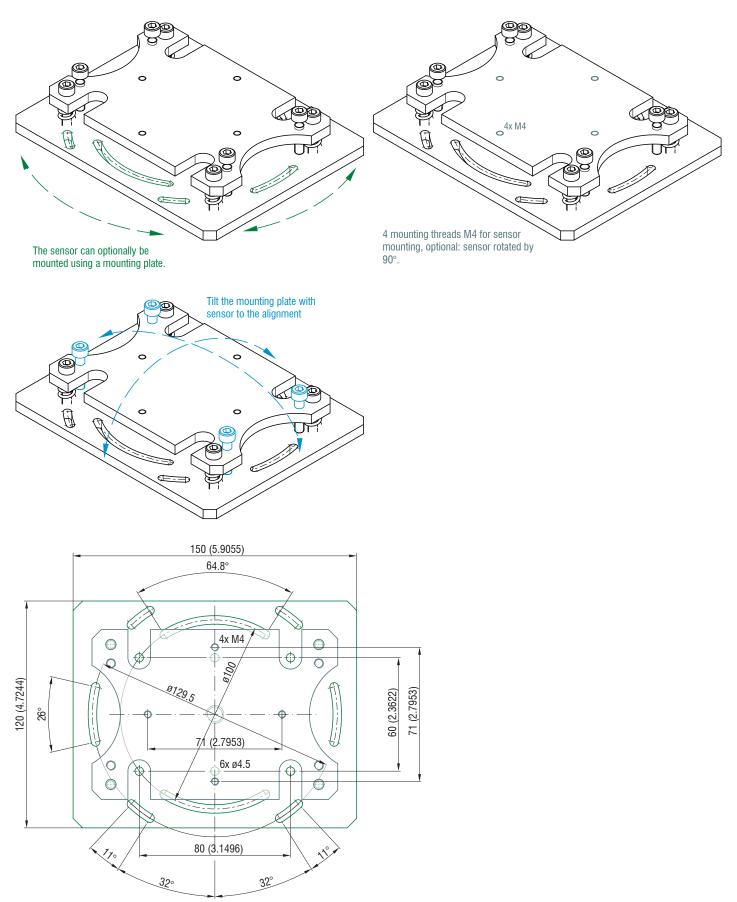
Abb. 32 Dimensional drawing mounting plate ILR-MP3800, dimensions in mm (inches, rounded off)
