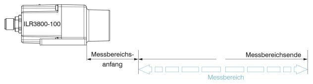
Abb. 8 Housing edge as point of reference for start of measuring range
