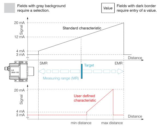
Abb. 24 Scaling the analog signal
