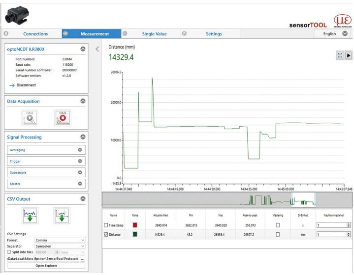
Abb. 17 Measurement view in the sensorTOOL program
