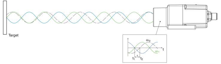
Abb. 2 Evaluation of the phase displacement for determining the distance
