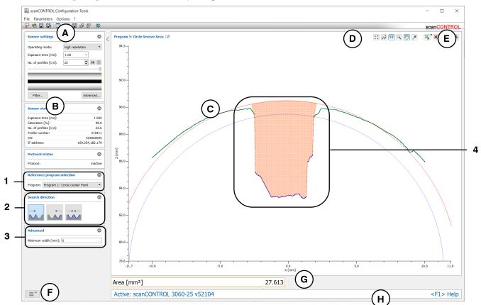
Fig. 4.54: "Circle Groove Area" measuring program
