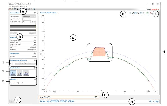
Fig. 4.49: "Circle Seam Area" measuring program
