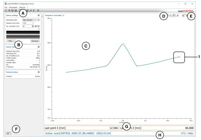
Fig. 4.5: "Last Point" measuring program
