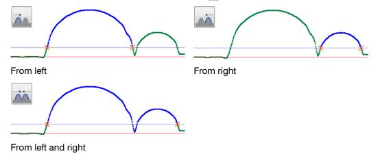
Fig. 4.26: Algorithms for the search direction
