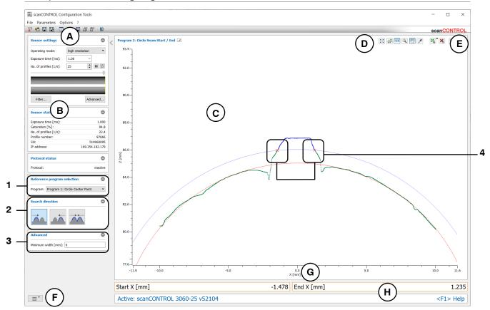
Fig. 4.46: "Circle Seam Start/End" measuring program
