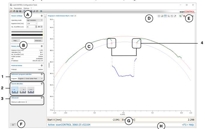
Fig. 4.51: "Circle Groove Start/End" measuring program
