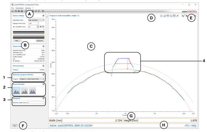
Fig. 4.48: "Circle Seam Width/Height" measuring program
