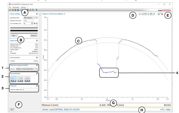
Fig. 4.52: "Circle Groove Minimum" measuring program
