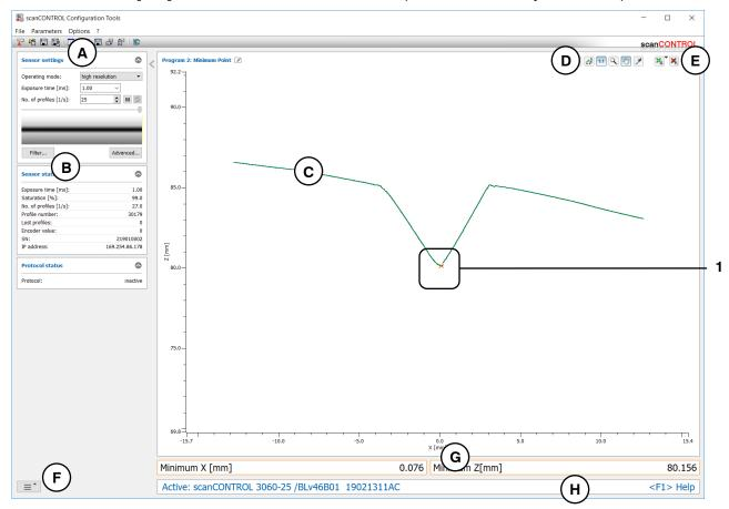
Fig. 4.3: "Minimum Point" measuring program
