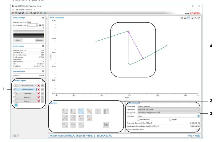
Fig. 5.2: "Result Combination" view - defining signals for calculation
