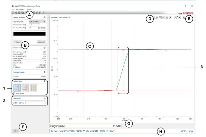
Fig. 4.17: "Step Height" measuring program
