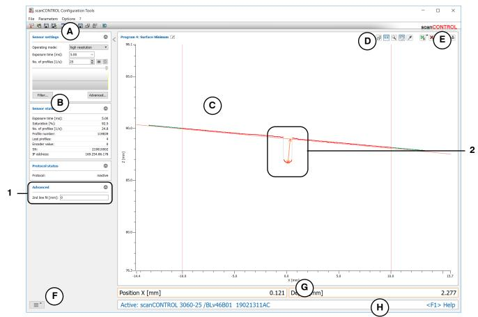
Fig. 4.24: "Surface Minimum" measuring program
