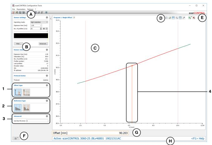
Fig. 4.14: "Single Offset" measuring program
