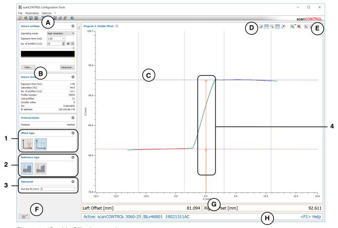
Fig. 4.15: "Double Offset" measuring program
