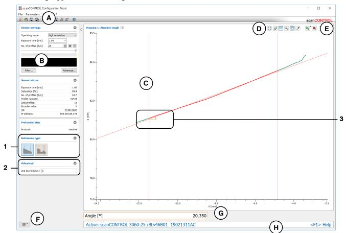
Fig. 4.7: "Absolute Angle" measuring program
