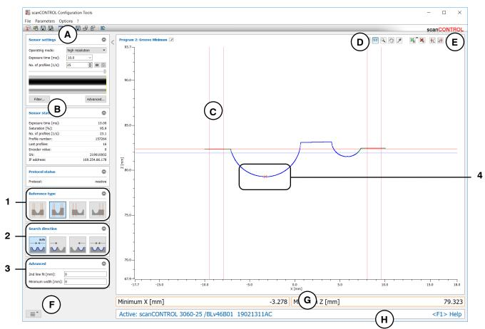
Fig. 4.33: "Groove Minimum" measuring program
