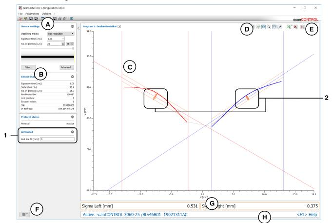
Fig. 4.22: "Double Deviation" measuring program
