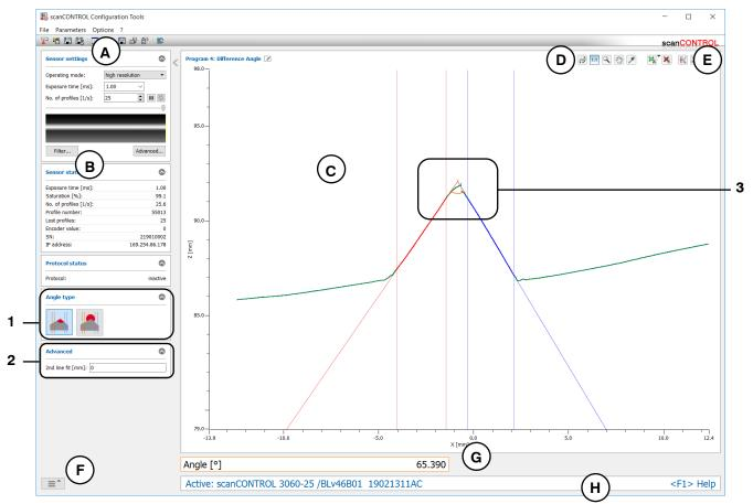
Fig. 4.10: "Difference Angle" measuring program
