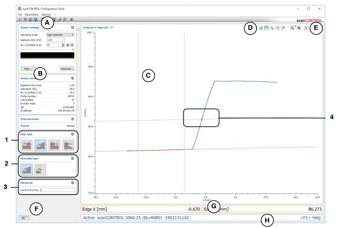
Fig. 4.18: "Edge Left" measuring program
