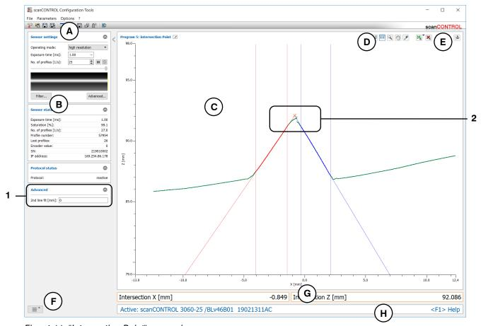
Fig. 4.11: "Intersection Point" measuring program
