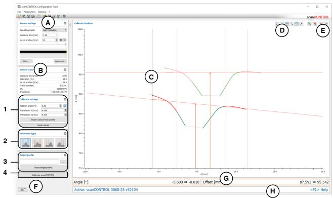
Fig. 4.59: "Calibrate Position" program
