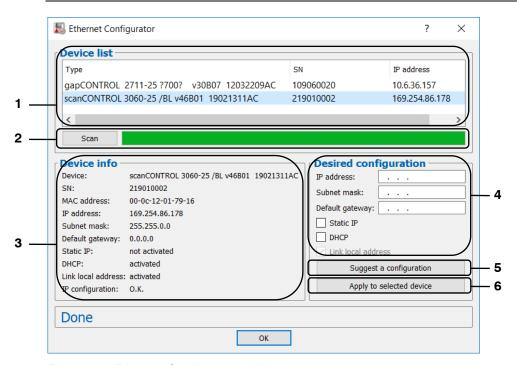
Fig. 3.75: "Ethernet Configurator" dialog
