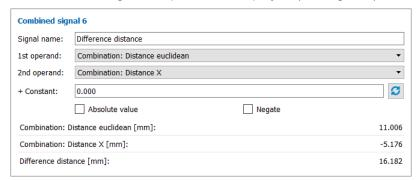
Fig. 5.6: Defining a new signal for calculation - step 3
