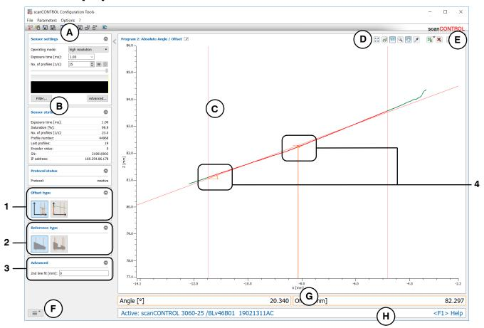
Fig. 4.8: "Absolute Angle/Offset" measuring program
