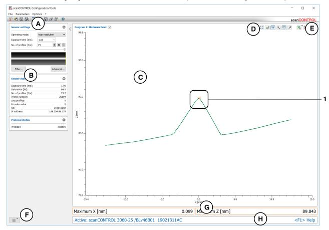
Fig. 4.2: "Maximum Point" measuring program
