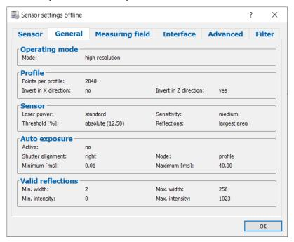
Fig. 3.20: "General" tab sheet in the "Sensor settings offline" dialog
