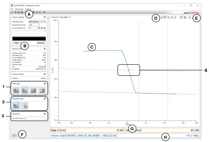
Fig. 4.19: "Edge Right" measuring program
