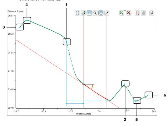
Fig. 3.51: Possible candidates for the anchor point
