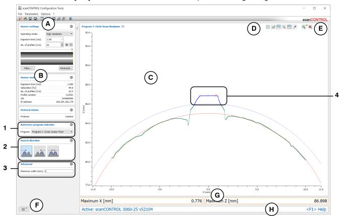
Fig. 4.47: "Circle Seam Maximum" measuring program
