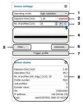
Fig. 3.12: "Sensor settings" input field
