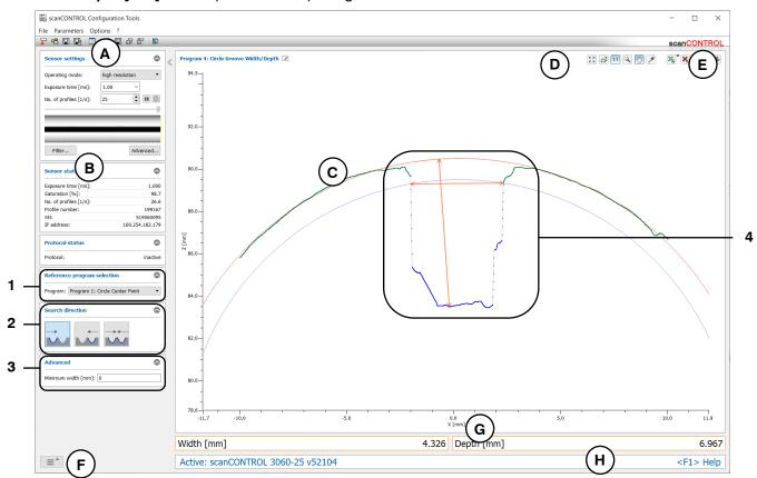
Fig. 4.53: "Circle Groove Width/Depth" measuring program
