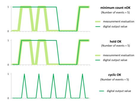
Fig. 6.7: "Digital port counter" example
