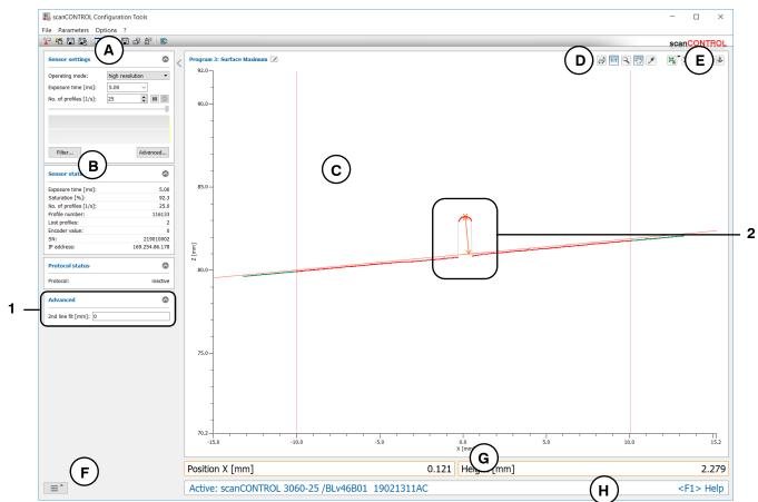
Fig. 4.23: "Surface Maximum" measuring program
