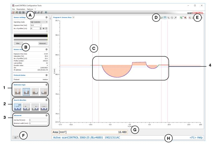
Fig. 4.35: "Groove Area" measuring program
