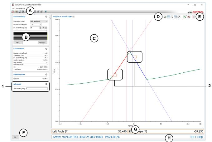
Fig. 4.9: "Double Angle" measuring program
