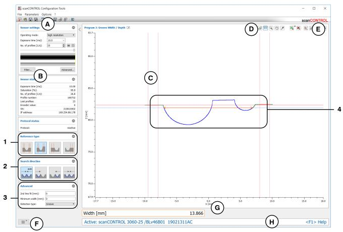
Fig. 4.34: "Groove Width/Depth" measuring program
