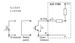
The switching inputs for laser on/off and setting masters/mid-point are similarly wired. Connect pin 9 with pin 6 in order to activate the laser. If the connection is released, the laser is deactivated.
