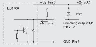
The transistor T is conductive in the active state. The switching outputs are short-circuit-proof.
