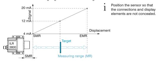
Start of measuring range, minimum distance between sensor and target
