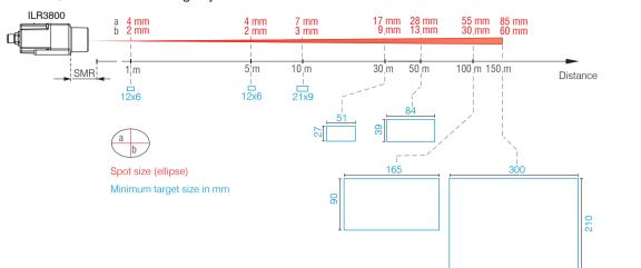
Fig. 2 Laser spot dimensions and size of measuring object depending on the distance
