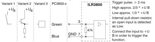
Fig. 4 Basic circuit for multi-function input
