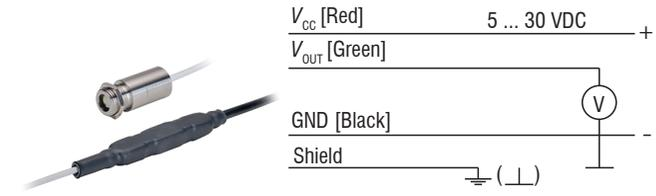
Pin assignment voltage output
