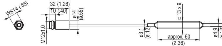
Dimensional drawing thermoMETER SE-SF15-S05-C05, dimensions in mm (Inches, rounded off)
