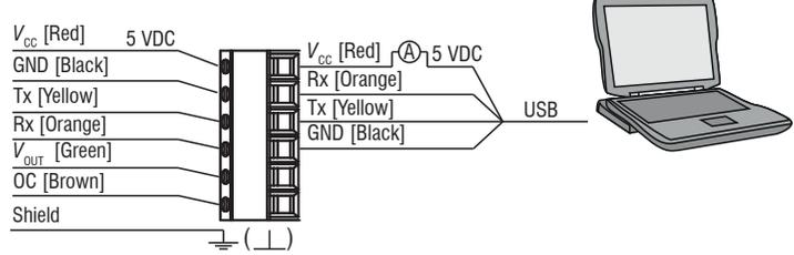
Pin assignment analog and digital output combined
