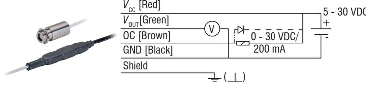
Terminal assignment open-collector output
