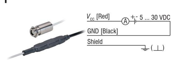
Pin assignment current output as two-wire sensor
